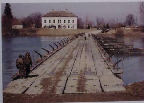
The Hungarian Engineers' PMP (Pontommo Mostovj Park, former Soviet Pontoon Bridge Set) across the River Sava.
