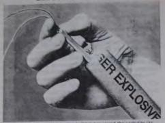
Insert detonator and take two half hitches round the cartridge (as shown in Fig. 2)
