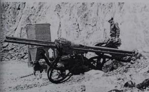
The AT-480 dust collector, available with YD-90 drifter or DHD-09 Down-hole drill, uses only 2 m<sup>3</sup>/min (70 cfm) of 7 kg/cm<sup>3</sup> (100 psi) air.
