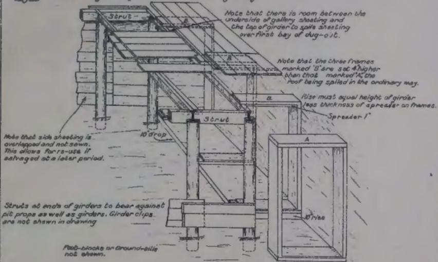
**Fig. 2.** Method of waterproofing dug-out.
