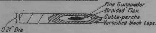
Fig. 2. Safety fuze. Scarfed cut unsevered.
