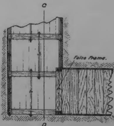
*Fig. 4. Breaking out from shaft.*
