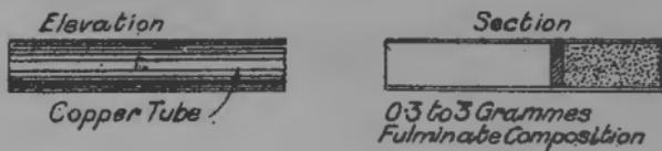
Fig. 2. Connecting Detonator to Safety Fuze.
