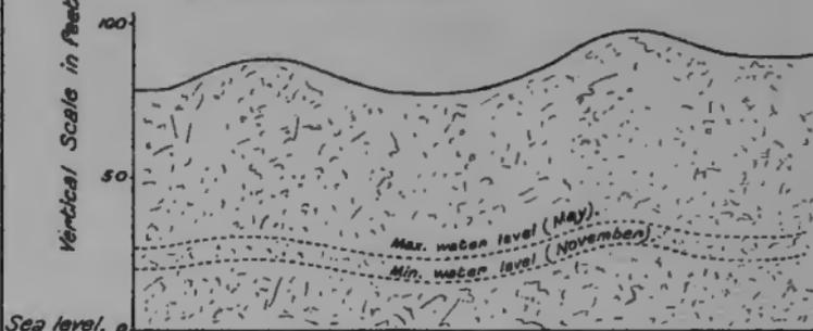
Fig. 2. Water under pressure.
