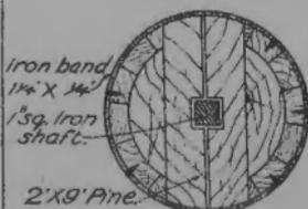
Fig. 2. Enlarged Section thra. A. B.
