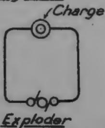
Fig. 4. Circuit with bare wire return.
