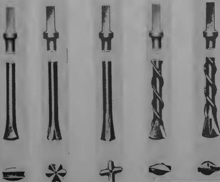
FIG. 2.—BITS SHOWING CUTTING EDGES.
