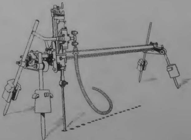
**FIG. 2. QUARRY BAR MOUNTING.**
