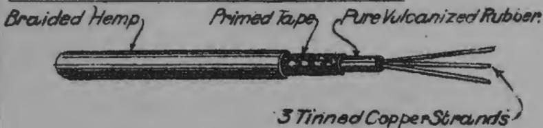
Fig. 3. Circuit insulated throughout.
