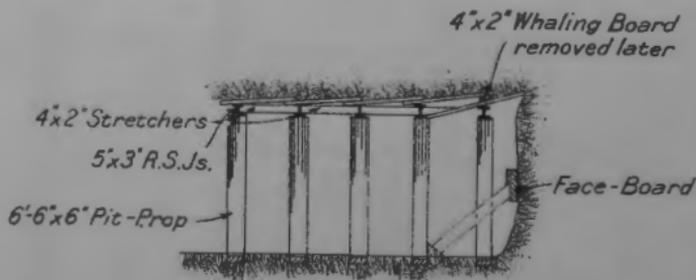
Fig. 3. With Pit-Props & R.S.J.s.
