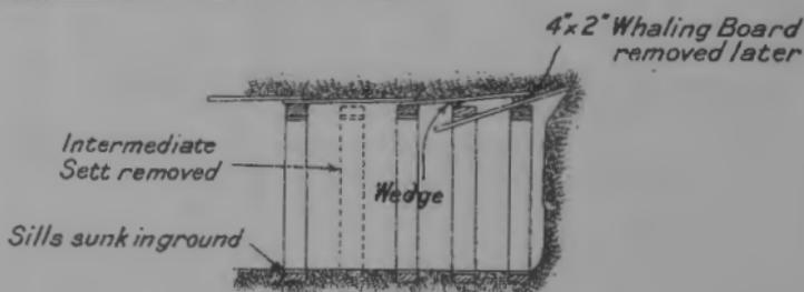
Fig. 2. With Intermediate Sett.
