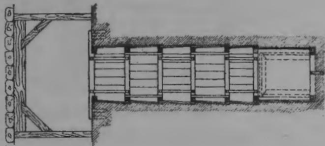
METHOD OF SINKING BY SPILING.
