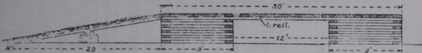
Double Platform constructed of Sleepers and Rails.
