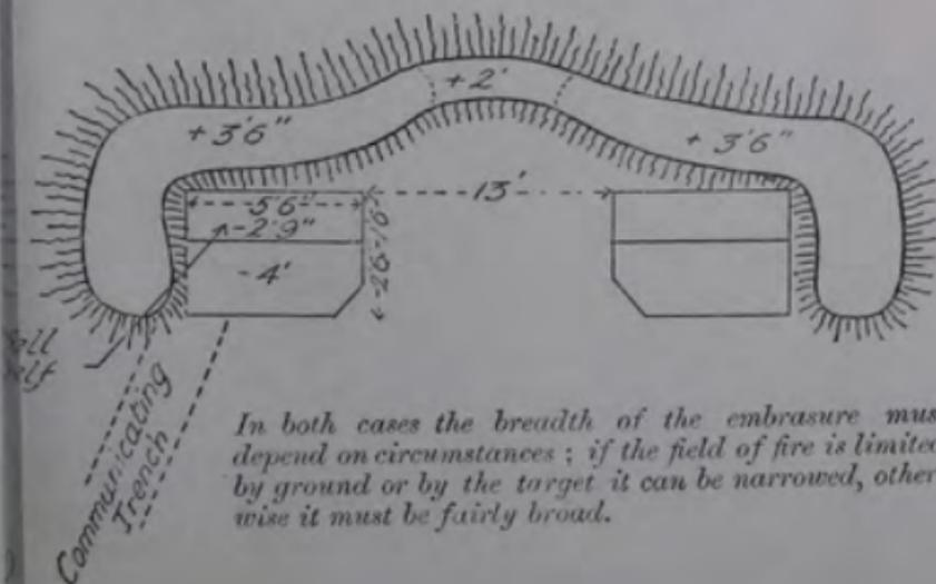
In both cases the breadth of the embrasure must depend on circumstances; if the field of fire is limited by ground or by the target it can be narrowed, otherwise it must be fairly broad.
