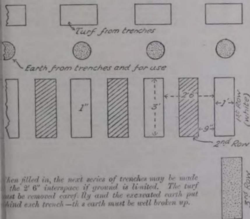
When filled in, the next series of trenches may be made in the 2' 6" interspace if ground is limited. The turf must be removed carefully and the excavated earth put behind each trench — this earth must be well broken up.
