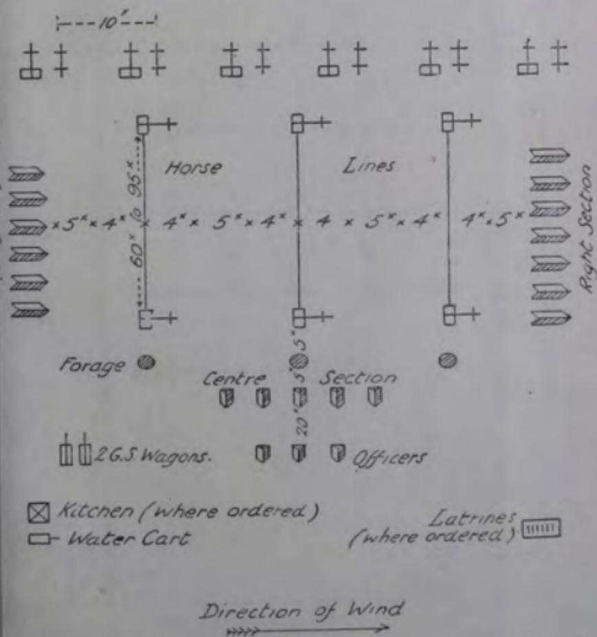
the horses of each section are fastened to one rope, using both sides of the rope. 5 feet between horses, and end horses 5 yards from vehicle.
