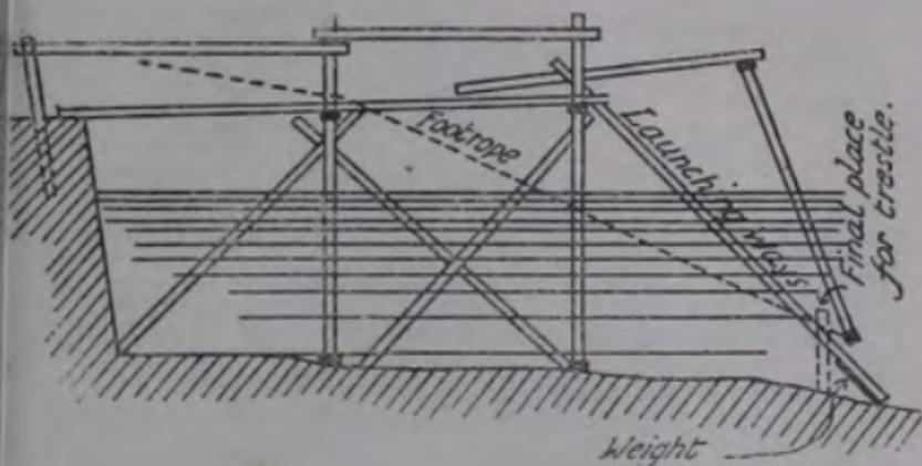
Fig. 2.—CANTILEVER BRIDGE.
