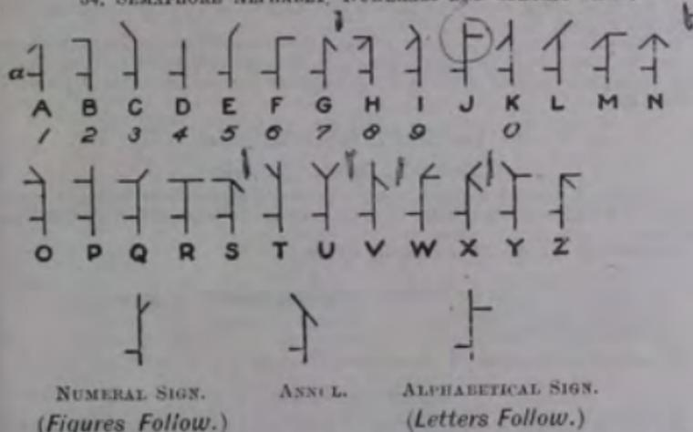
The small arm at *a* is called the "Indicator," and shows the side from which the Alphabet or signs commence; the signaller, when working a fixed semaphore, is sometimes not visible, and the indicator is necessary because his back may be toward the reader. It also often happens on board ship that a semaphore signal is being read from both sides at the same time, and unless the indicator was used the reverse letters might be read, e.g., K for V.
