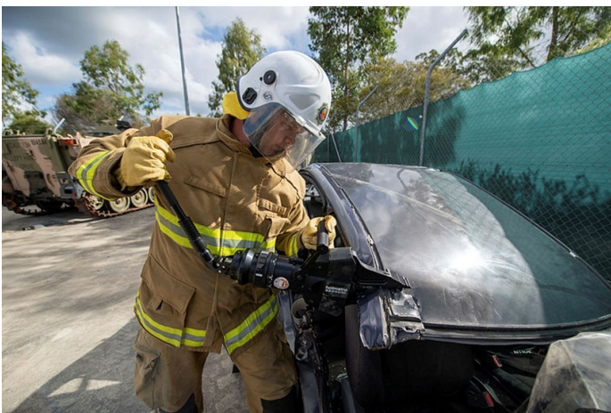
Figure 1: Sapper Domjahn uses a spreader and cutter tool from the new Light Rescue Kit
