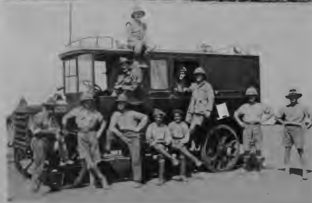
Lorry Wireless Set, mounted on a Daimler chassis. During the greater part of the campaign the Second Squadron (English) had a number of these on duty at various L. of C. points; afterwards several went to Persia to take over from the Squadron, while another was transferred to us for use at Shargat as control station during the latter part of the Mosul operations. In February it took up duty at Baqubah, where this photograph was made.
