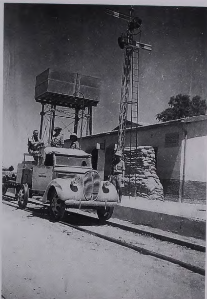
Right: A pick-up truck freshly converted to a rail patrol car.
