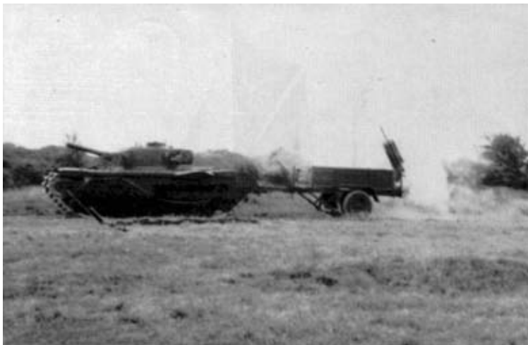
Giant Viper being fired from a Churchill AVRE
