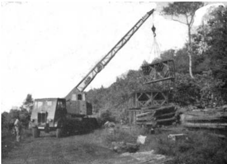
Coles 7-ton crane unloading stores in the field
