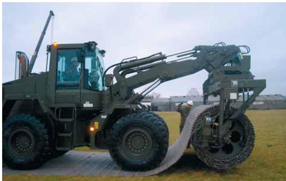
Figure 6 – Class 30 Trackway forms the perimeter track.
