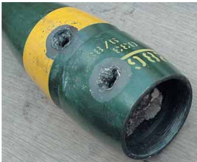
Plate 7 – UK 81mm Mortar Bomb: fuze ejected by firing water into the body.
