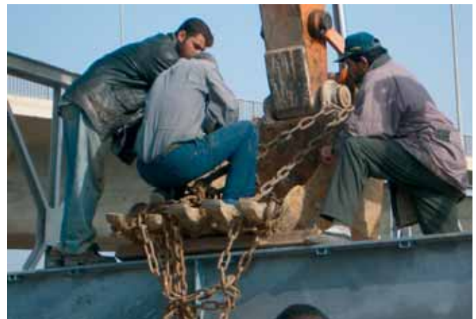
The excavator bucket being fixed to the rear transom on the tail.
