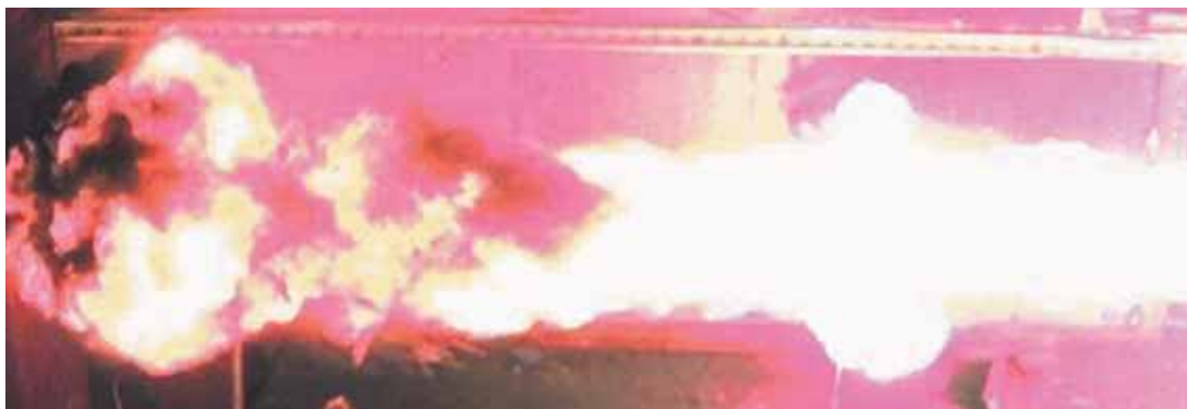
Plate 5 – High speed video of jet of burning magnesium emerging from a 37mm thick steel target
