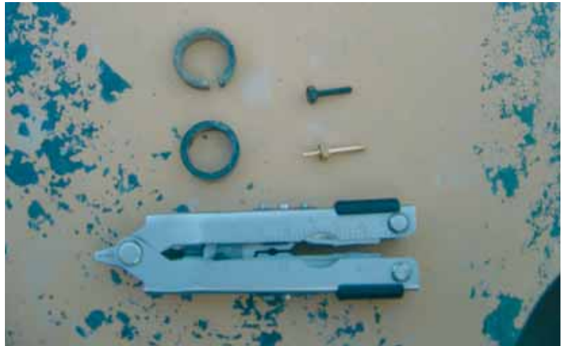
A broken (top) and new (bottom) O-ring and needle.
