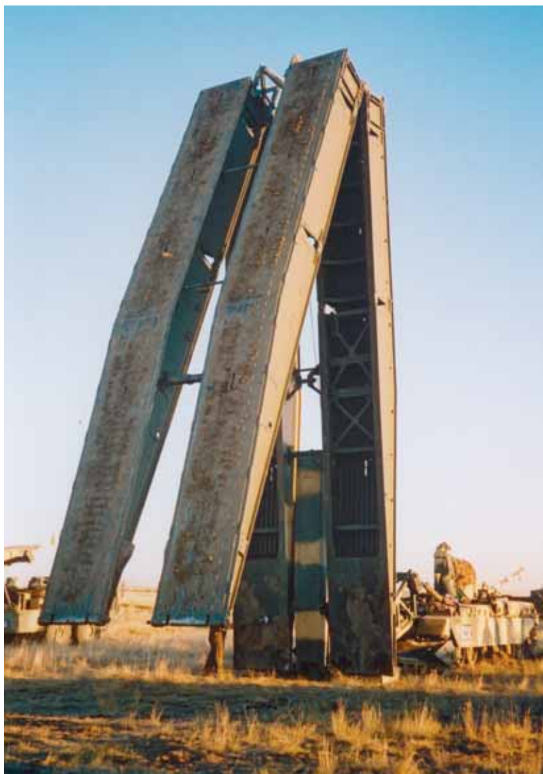
An AVLB launching a No 10 bridge during Ex Iron Anvil 03.
