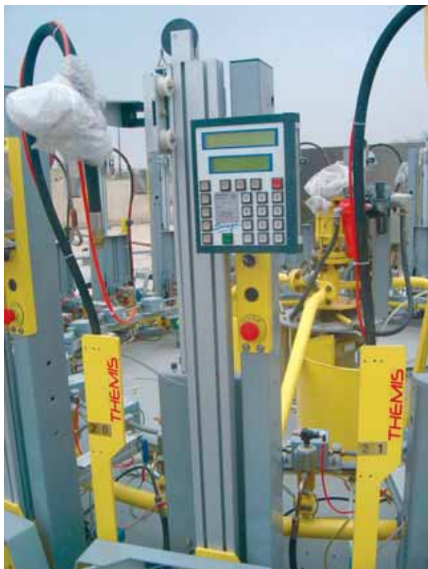
New automatic carousel bottling plant equipment being installed at Arabian Gulf Plant.
