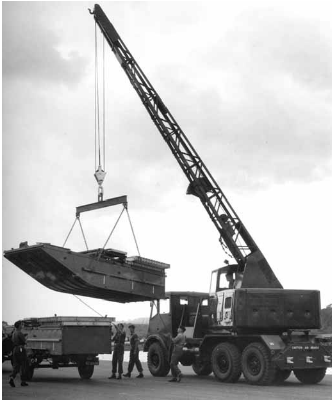
A Coles Bridging Crane lifting a LAFB Pontoon.
