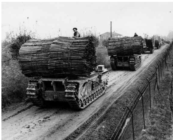
Figure 8 – Two Churchill AVREs carrying fascines are seen in the above photograph moving up to the front line. The fascines are held in front of the Churchill's turret and are mounted on a wooden cradle fitted to the front of the tank. As the tank driver had no forward view, the tank commander, or other crew member, is guiding the tank along the road. He is, presumably, standing on the tank's turret. The tank's main gun would be pointing to the rear or to the side as if it was a howitzer. Two ARKs can be seen behind the two fascine-carrying AVREs.
