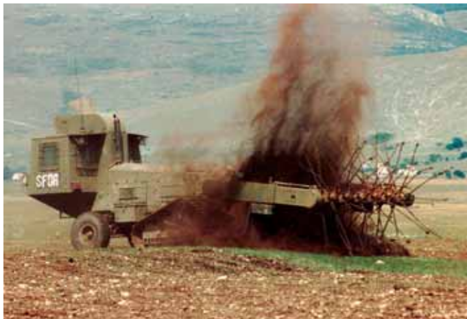
Mechanical Clearance Equipment – Large purpose built flails.
