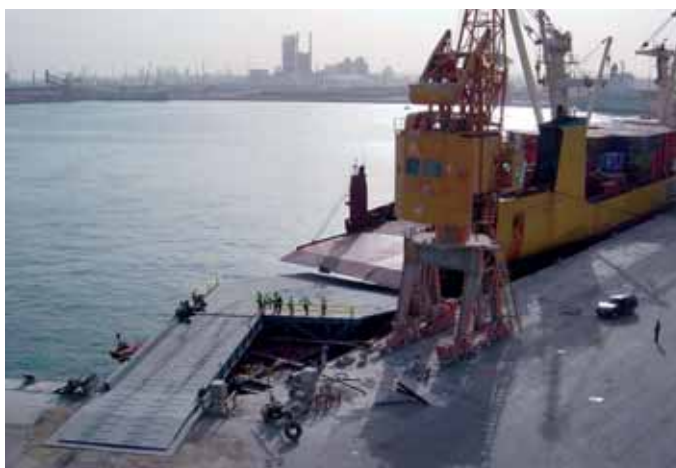
Ferry docking with the RoRo Linkspan enabled through the Staff Corps in Kuwait.
