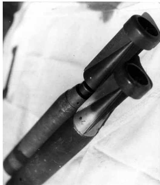
Brace of German 1kg incendiary bombs with the top example’s tail exposed to reveal hidden explosive charge.
