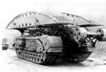
Figure 2: Churchill "Jumbo" bridgelayers – robust, practical and effective in battle.
