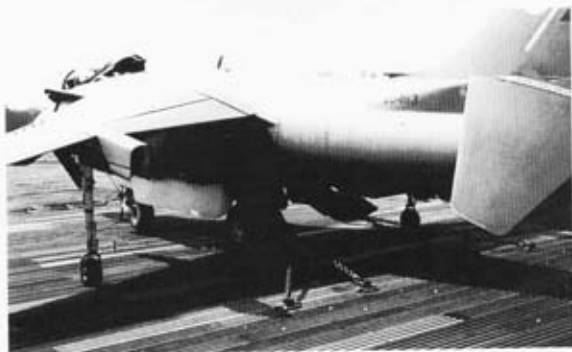
Rear detail of Harrier correctly anchored and ready for testing.
