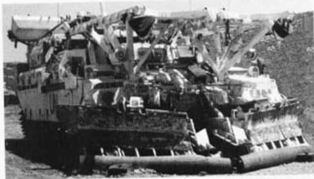
Trialling an adapted hard surface mine clearance device on an AVRE.
