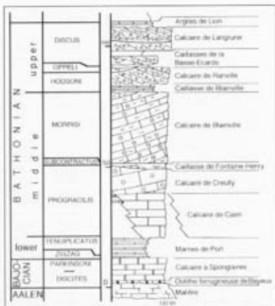
Figure 7. Part of the Middle Jurassic sequence of Normandy (somewhat generalized), to be found between Bayeux and Caen. Stage and ammonite zone names are to the left, formation names (in French) to the right. Total thickness is some 100m, mainly limestone (calcaire) but with some clays (argilles) or marls (marnes). (From Rioult et al, 1991).
