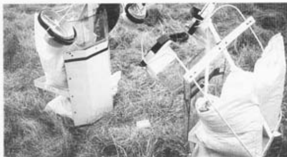
Blast testing of Development Technology Unit designed shields and visors under RE supervision.
