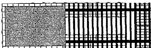
Figure 10. Stripped down baskets are placed on top of the crossovers. Plastic sheeting is laid over the top of these and secured with sandbags.
