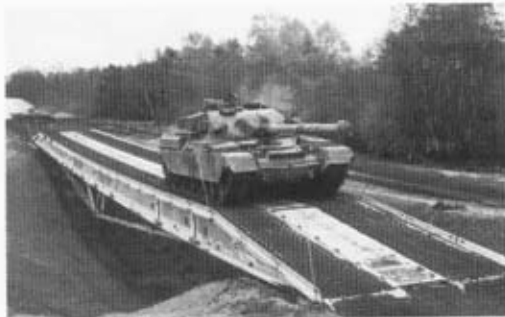
A tank crossing the MLC 70(T) 56m long LSB during testing.
