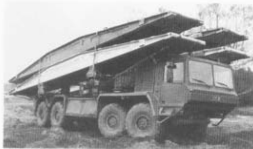
2 x No 12 Bridges on a tank bridge transporter (TBT).
