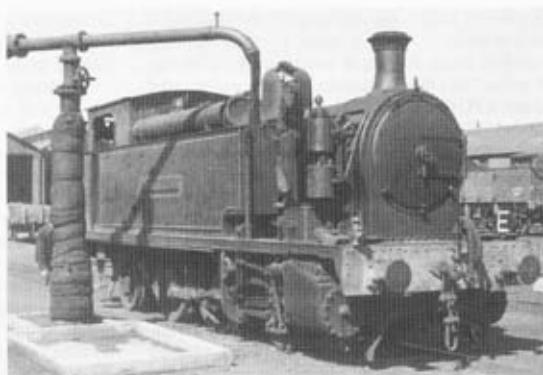
No 203 Sir John French takes on water at Longmoor. Note the insulation of the water column against frost, also the rerailling ramp behind the headlamp. "Sir John" had a long and successful life at Longmoor during and between World War One and Two. The locomotive had numerous fittings to facilitate training, including the Weir steam feed pump and outside Walschaerts valve gear.
