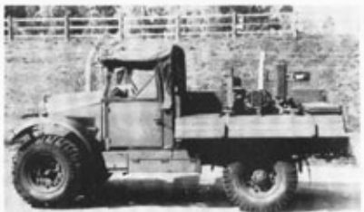
The ubiquitous Morris Commercial compressor truck with its two-cylinder, two-stage air-cooled compressor.
