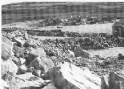
Photo 5. Military quarrying, Falkland Islands. (Photo courtesy of the Librarian, Technical Information Centre RE.) Aggregates have often been required in large quantities during or after military operations, primarily for road or airfield construction. Geological factors influence both siting and development of quarries.
