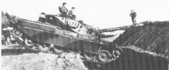
Photo 4. Trial antitank ditch. Geologically-related factors combined with weather conditions strongly influence cross-country mobility, and the position, nature, and speed/means of construction of earthworks designed to impede it.
