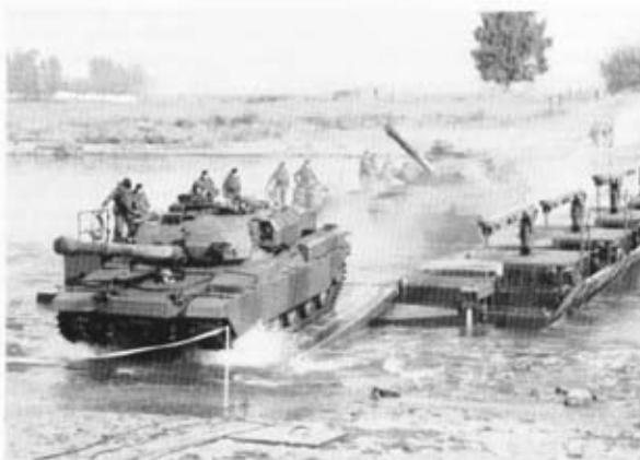
Two tanks leaving a four rig M3 ferry which had just crossed the Weser in 70 seconds.
