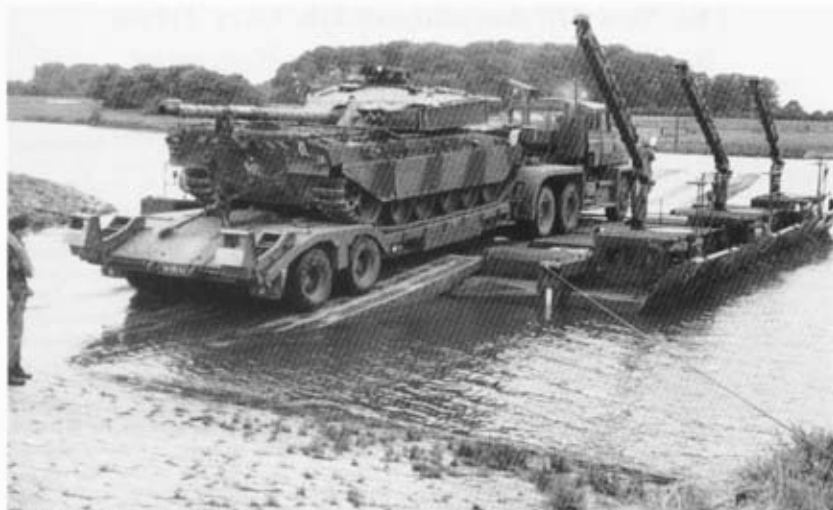
A three rig M3 ferry loading a tank transporter and Challenger tank at MLC 100(W). Taken during trials at Barmse on the Weser, October 1991.
