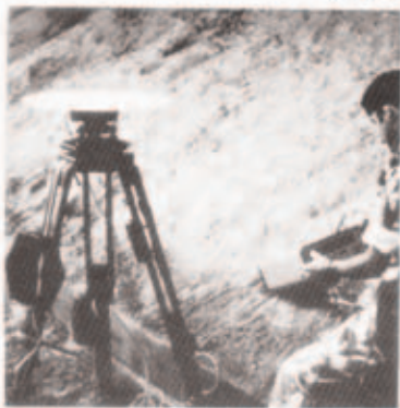
Field Survey support for Royal Artillery. A Global Positioning System Trimble 4000 SST set in use in Northern Saudi Arabia
