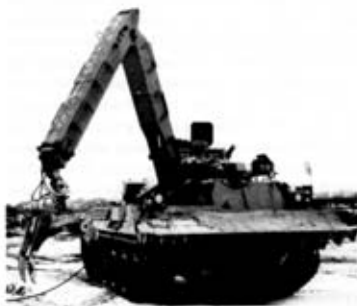
Front view of EBG showing working arm deployed with grab attachment. Scarifying teeth can be seen on underside of dozer blade.
