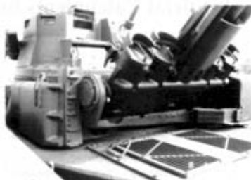
Close-up of armament. Central tube is demolition round launcher with two mine launcher tubes on each side.
