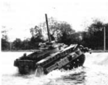
EBG exiting water obstacle with snorkelling tube deployed.
