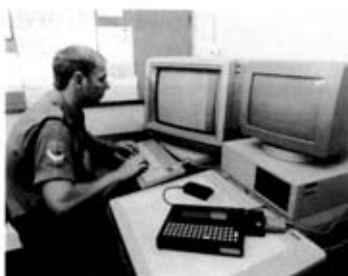
Field observations are transferred directly to the main computer which automatically produces site plans.
