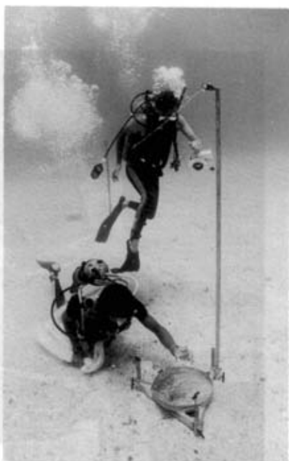
Photo 3. Divers testing the mercury mirror, a photogrammetry aid used to ensure vertical photos.
