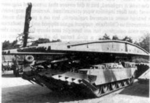
Photo 2. Chieftain AVRE, with mine-plough mounted, carrying a Number 9 tank bridge.
