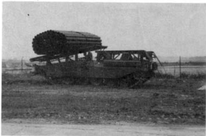
Photo 3. AVRE at speed; having launched one fascine the second is ready and will be covered by the Class 60 trackway being dragged behind. Note the tilt of the hamper achieved by the rear rams being fully extended and the front ones fully retracted.
