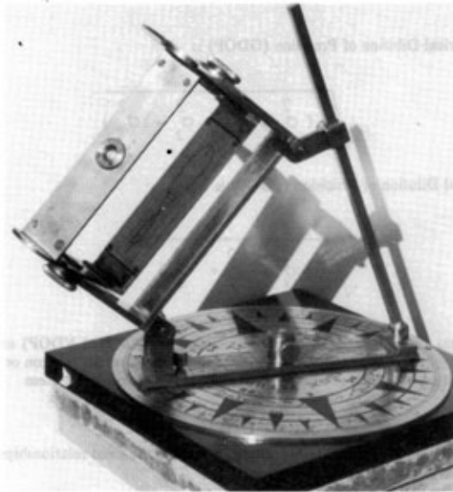
Photo 1. General view of the phoeboscope. Note the bright spot projected by the lens of the gnomon onto the shadow plate.
