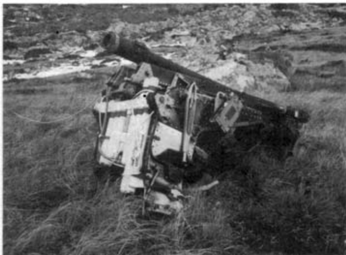
Photo 2. The rear of the two Martin Baker ejector seats with propellant cartridges.
