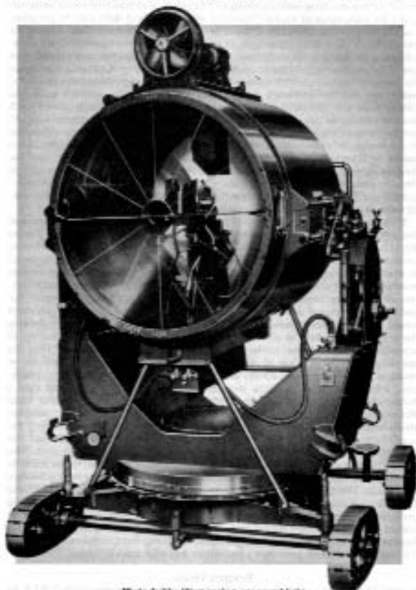
Photo 4. The Wien carbon arc searchlight
