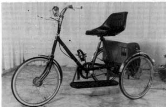
Photo 2. The Uni-pedal Batri-trike fitted with a special seat for a Disabled Person whose balance is impaired. Note the "stirrup" fitted on the right pedal. Production models now all have a luggage carrier fitted
