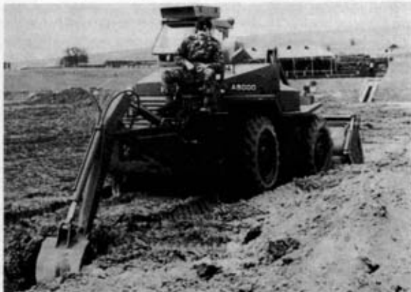
Photo 3. Back-actor mounted on Light Wheeled Tractor
