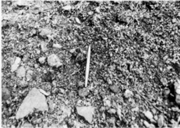
Photo 1. The type of soil on which the hydro-spraying was attempted. Note the coarseness of the material
