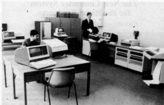
Photo 1. The Hewlett Packard System 1000/45. Showing the main console with, L to R, the console keyboard, the high quality printer plotter and the 180cps printer all in the background. Two of the four terminals are clearly seen in the foreground.
