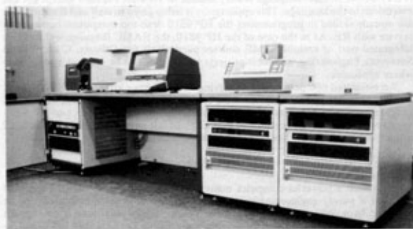
Photo 2. The main console unit, with the entire memory and control circuitry housed in the left-hand pedestal, and the two 20 million character disc stores on the right.
