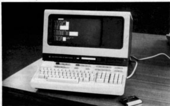
Photo 3. The graphics terminals have a refreshed display so providing zoom, pan and scrolling of 6,000 letters of text. A mini-cartridge tape capable of holding 110,000 characters is shown to the right. Each terminal will hold two of these cartridges.
