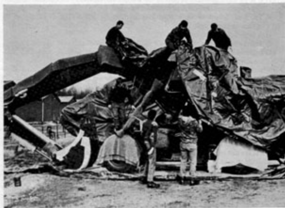
Photo 4. A percentage of the squadron plant is permanently stored on the RAF airfield. Here an Atlas excavator is being installed in its protective envelope.
