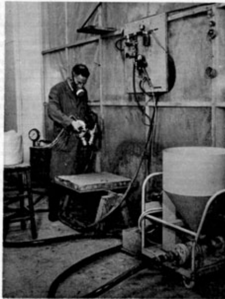
Photo 1. The spraying rig and vacuum mould.
