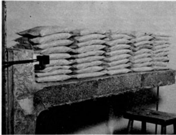
Photo 6. "Breeze block" beam under load.
