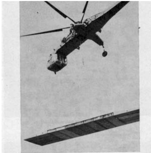
Plate 2. CH 54A Carrying 52 ft CI 16 (APB) Bridge complete.
