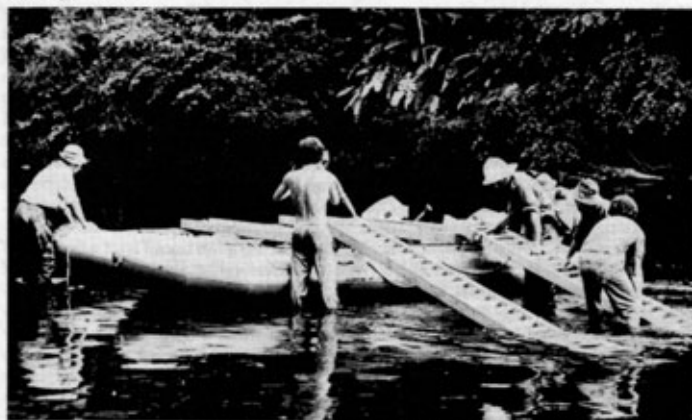
Plate 7. The M650 Avon Raft, built by Avon Ltd and CEP, being erected on the Tuira river, note MEXE ladders used for decking and ramps. Special Nylon load lok straps were used to hold it all together.
