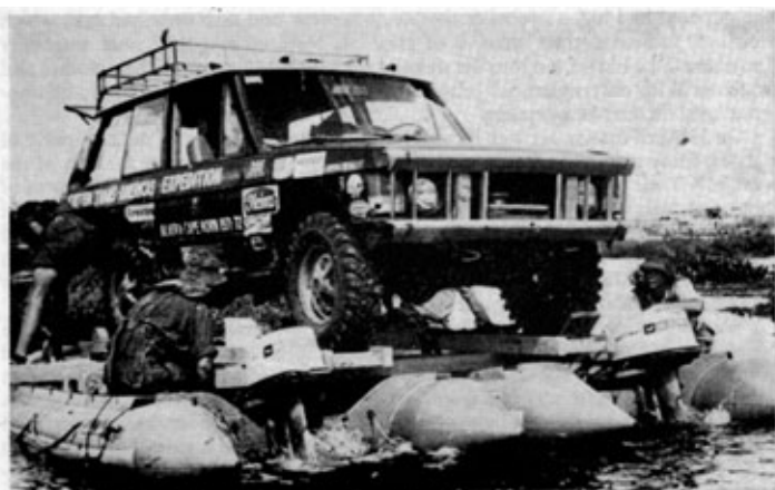
Plate 8. Assault on the Great Atrato Swamp. The Avon raft with MEXE ladders as deck and ramps. Note Colombian Navy Gunboat that was Expedition HQ for the assault in background.
