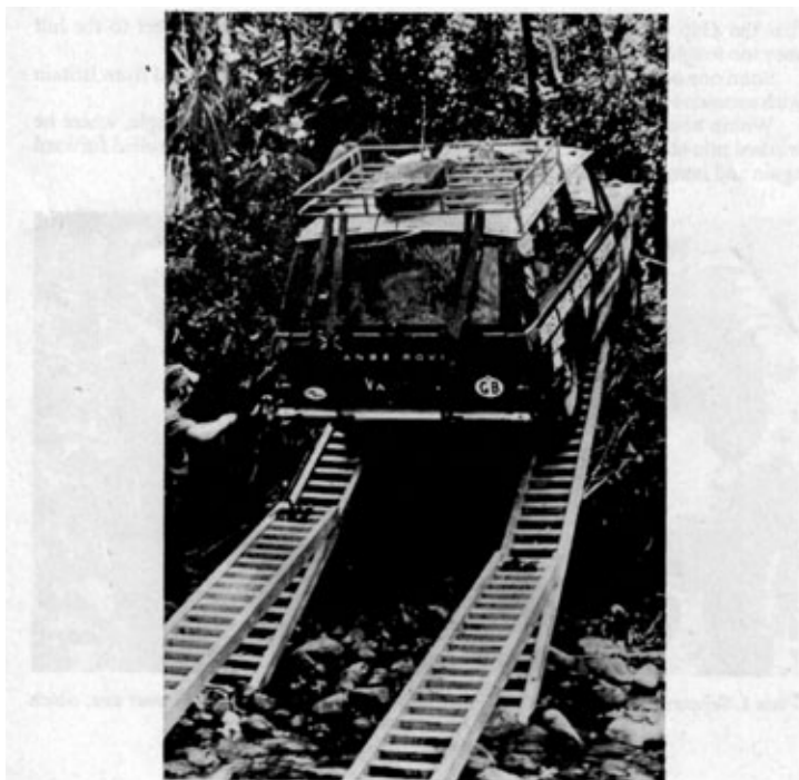
Plate 3. MEXE ladders and load lok straps used to get Range Rover up a 5 ft vertical bank.
