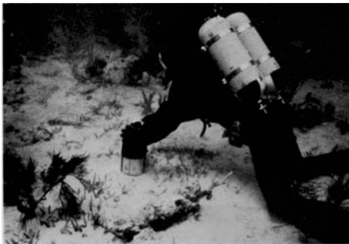
Plate 2. CD11 with Macaroni tin for air gap. A diver holds the charge down while another brings sand bags to fix the charge
