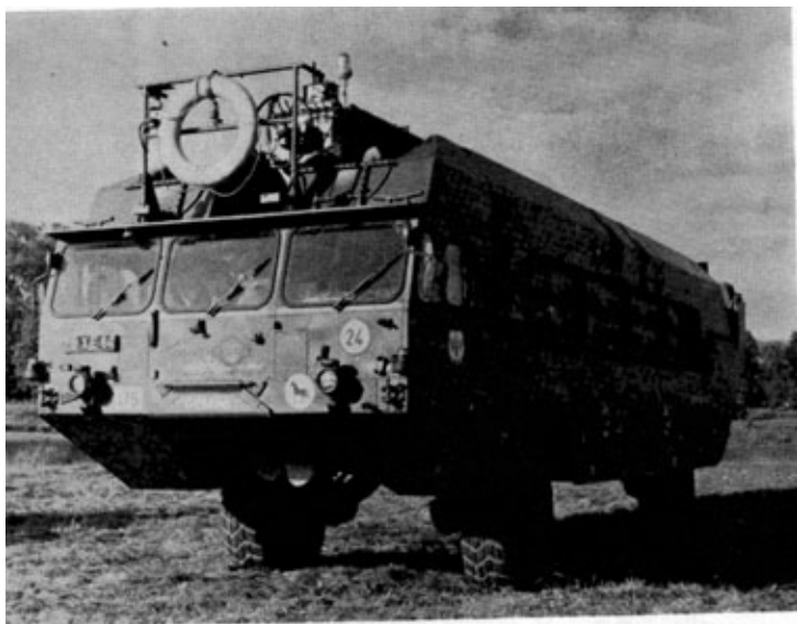
Photo 3. An M2 Amphibian. 10 feet wide, 37 feet long, weighing 22 tons with a crew of four
