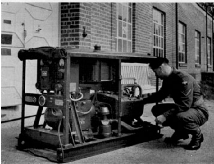
Fig. 2. 5 kVA generating set, single-phase 240V 50 Hz.
