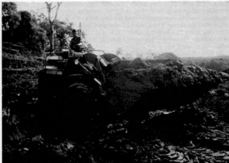
Fig. 9. Size 8 wheeled tractor with three cubic yard multi-purpose bucket—working well in extremely heavy going during wet monsoon.
