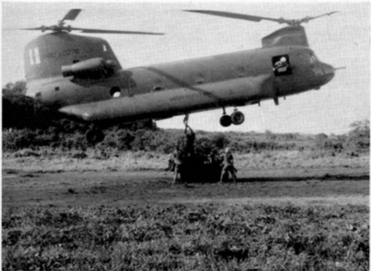
Fig. 5. CH 47 "Chinook" lifting Size O tracked tractor for transport to new helipad site.
