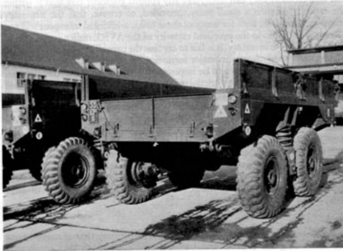
Photo. 5. The AVRE Trailer. The trailer has a capacity of 7\frac{1}{2} tons and an excellent suspension system (Note the heavy coil springs).
