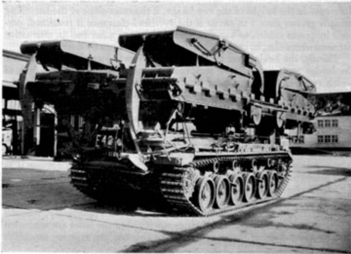
Photo. 2. The Centurion Ark (rear view). Note the rear stabilizer (just below the callsign board) which, when released to the ground, moves up and down on a ratchet to reduce rocking as vehicles cross the bridge.
