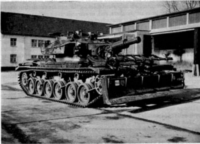
Photo. 4. The Centurion AVRE. The demolition gun, fascine cradle (just below the gun) and the dozer blade are clearly seen in this picture.
