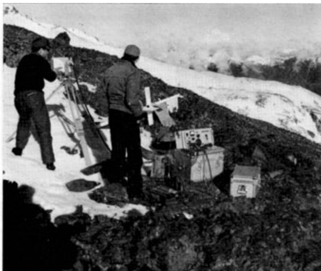
Photo 5. Observations at BP VII-2G, on the northern slopes of the Cerro da la Virgen, with a Wild Distomat by Senor Soria (Argentina) and Major Cepeda (Chile).
