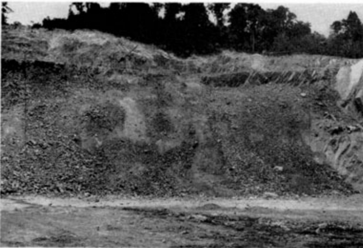
Photo. 4. The same quarry face after the blast, showing well fragmented rock. The frameworks for rain shelters for the explosive, when stacked on the bench top, on the working area to the rear of the bench can be seen still in place.
