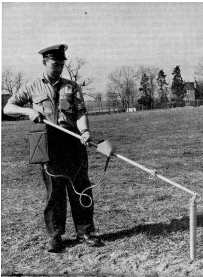
Fig 2. JSBDS Instructor with Forster 4013 surface locator.
