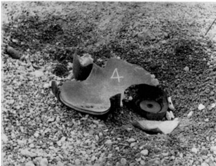
Fig 7. Result of attack on a 500 lb aircraft bomb
