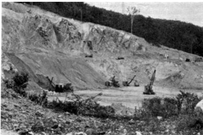
Photo. 1. This shows the granite nature of the quarry face (centre portion) before the blast. A drilling machine can be seen at the top of the picture on the bench top.
