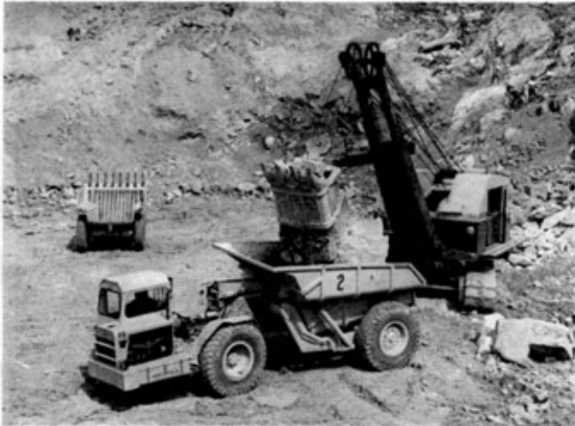
Photo 13. ARTICULATED DUMP TRUCK. Capacity 13 tons or 9 cu yds, unladen weight 13,500 lb. Maximum speed 28 mph.
