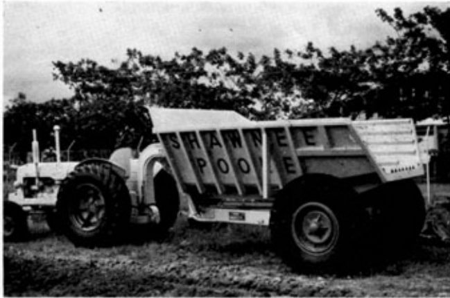
Photo 12. REAR DUMP HAULER. Capacity 10 tons or 7 cu yds, unladen weight 12,500 lb. Tractor Fordson Super Major. Maximum speed 14 mph.
