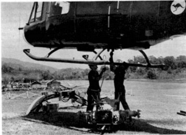
Photo 2. DISASSEMBLY. Gear box of Fordson Transatlant grader about to be heaved on to an Iroquois helicopter for extraction from a jungle airstrip. In the background is the grader main girder and a box of spare parts.
