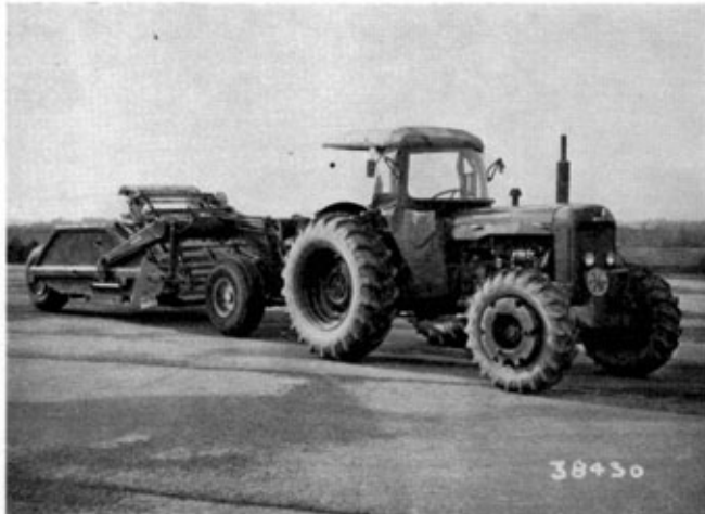
Photo 4. Johnson 40B, 4 cu yd self loading scraper towed by a Fergusson 65 tractor. The 11 cu yd version is similar.
