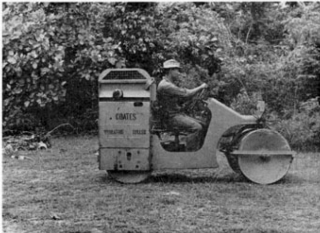
Photo 7. SELF-PROPELLED VIBRATING ROLLER. 32 ins 2½ cwt Coates roller—Stothert and Pitt made under licence in Australia.
