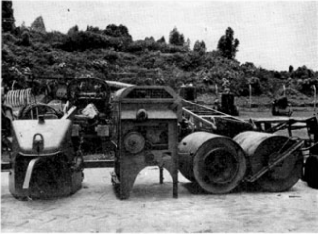
Photo 8. SEGMENTED VIBRATING ROLLER. The same 32 in self propelled vibrating roller segmented for carriage by Twin Pioneer.
