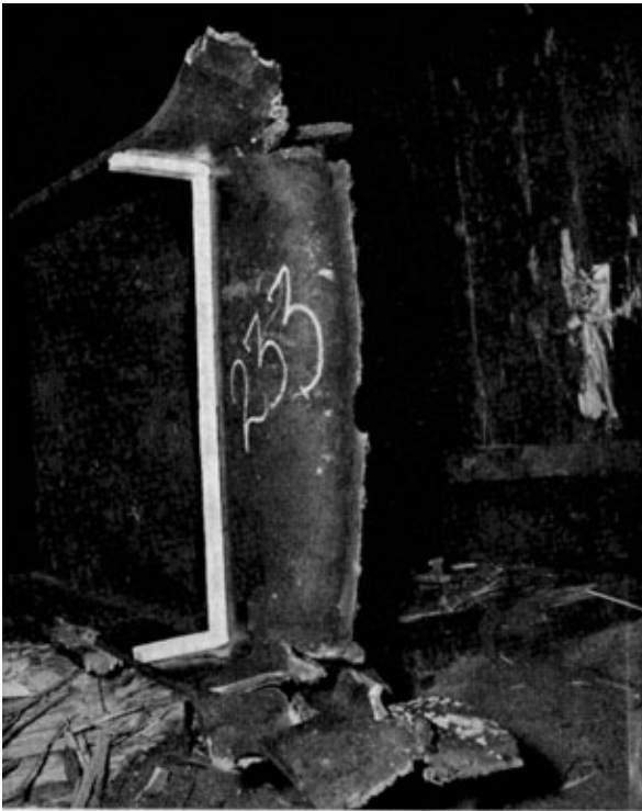
Photo 5. Ribbon charge on steel beam.
