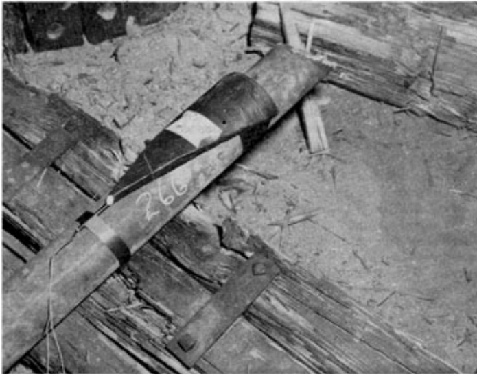
Photo 9. Saddle charge in place.
