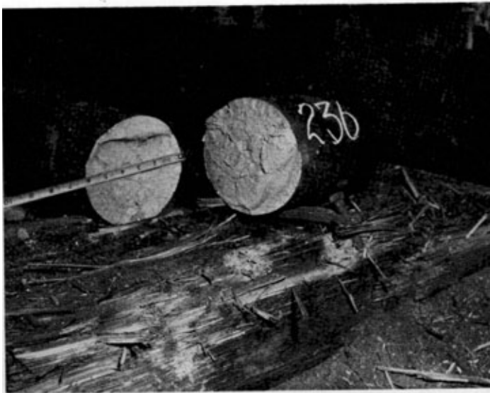
Photo 13. Results of initiating diamond charge by detonating card.
