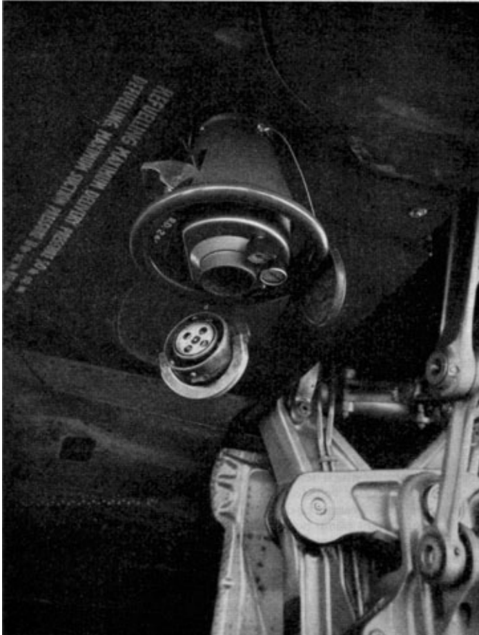
Photo 3. Hose-end pressure control valve fitted to aircraft fuel coupling, but with hose removed to show detail. The gauges show pre-set delivery pressure and actual fuel pressure
