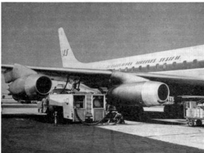
Photo 2. A DC8 supplied by a dispenser vehicle from a hydrant system. Note the two delivery hoses each supplying up to 210 gal/min. The aircraft can accept four hoses, two under each wing
