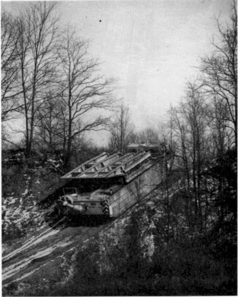
Photo 2. An end bay unit on a cross-country course. (The rear operator's pilot station is folded down into the hull just in front of the tubular backrest. Note the propeller in its stowed position; the hydraulic cylinders in the ramp; the male and female fittings on the lower layer on the deck; and the raised engine cooling system air vent between the aft capstan and the superstructure.)
