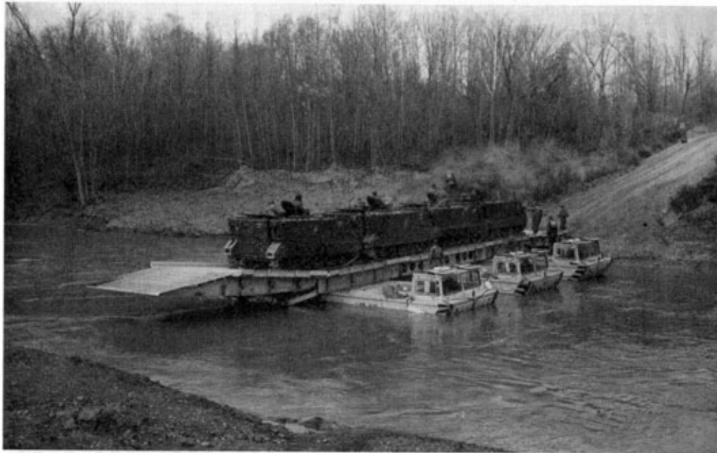
Photo 5. A three-bay raft (almost a bridge!) carrying four M113 APCs (approximately 44 tons total load.) (Note the raised kerbs; and the use of the ramp to support part of the rear APC. This raft is exactly 100 ft in length)
