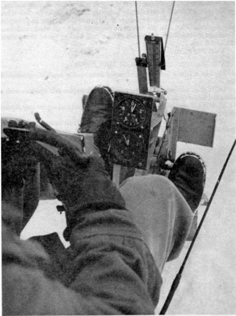
Photo 3. Pilots eye view. The throttle caliper control and the two electric switches referred to in the text can be seen on the cyclic stick.
