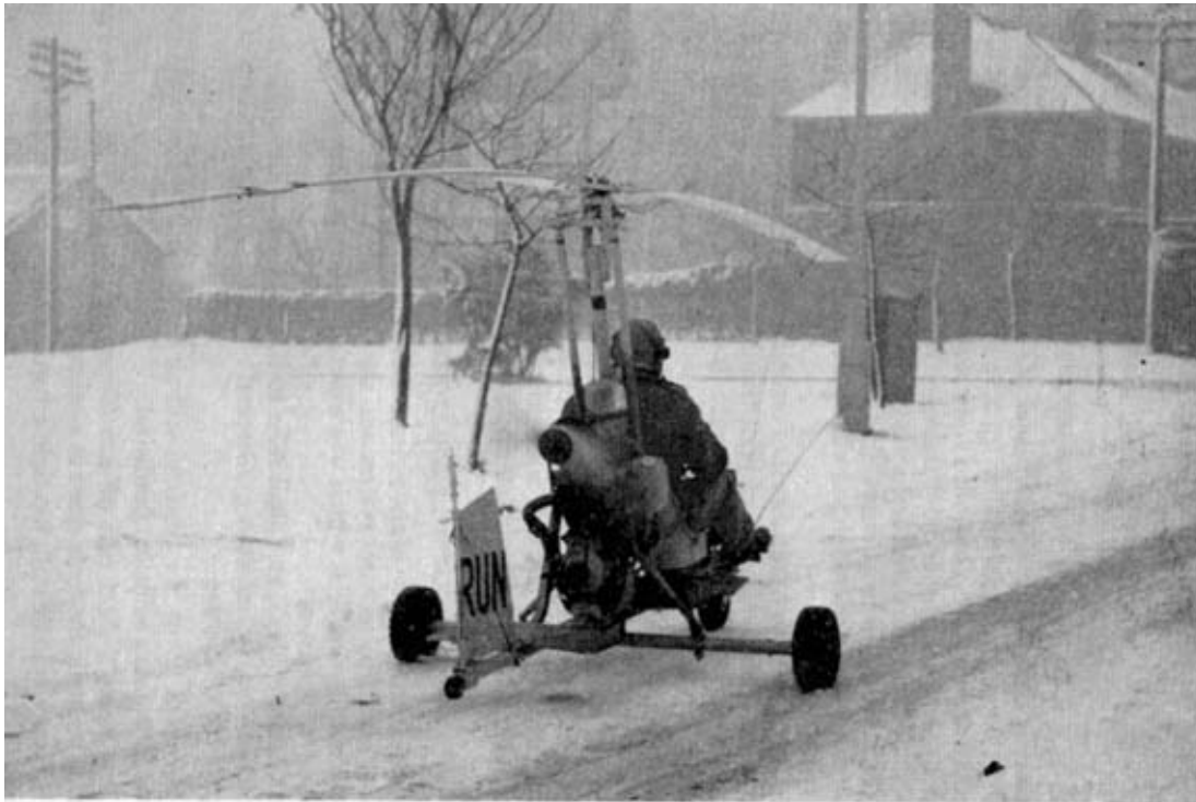
Photo 2. Transportation. With the blades either removed or secured fore and aft the recce-copter can travel on the road under the power of its pusher propeller.
