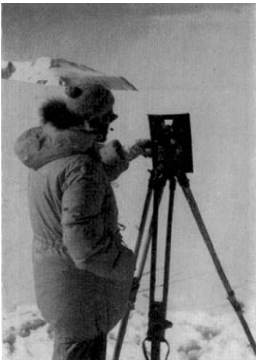
Photo 12. Surveying on the north bank of the Nimrod Glacier. A piece of leather is used to shade the theodolite from direct rays of the sun—thus obviating excessive temperature differences of the metal parts.
