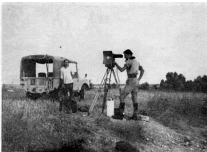
Photo 4. L/Cpl. Jago of the UK survey party observes a line in the Dhekelia area with a tellurometer set up over one of the boundary pillars. The party at the far end of the line is supplied by the Cyprus Department of Lands and Surveys.
