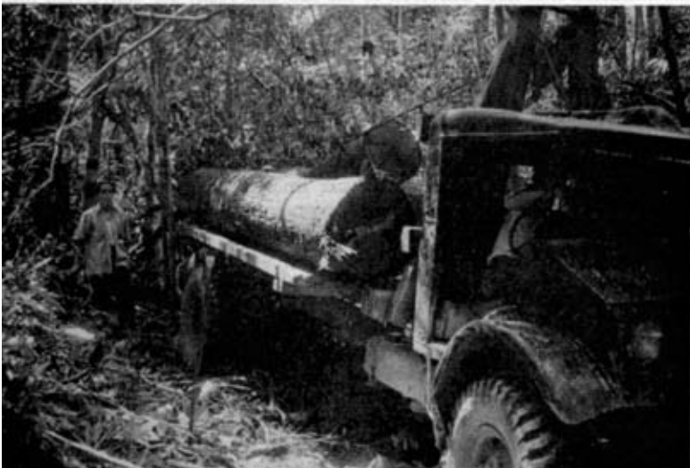
Photo 2. Winch loading a logging lorry Ulu Trenganu.
