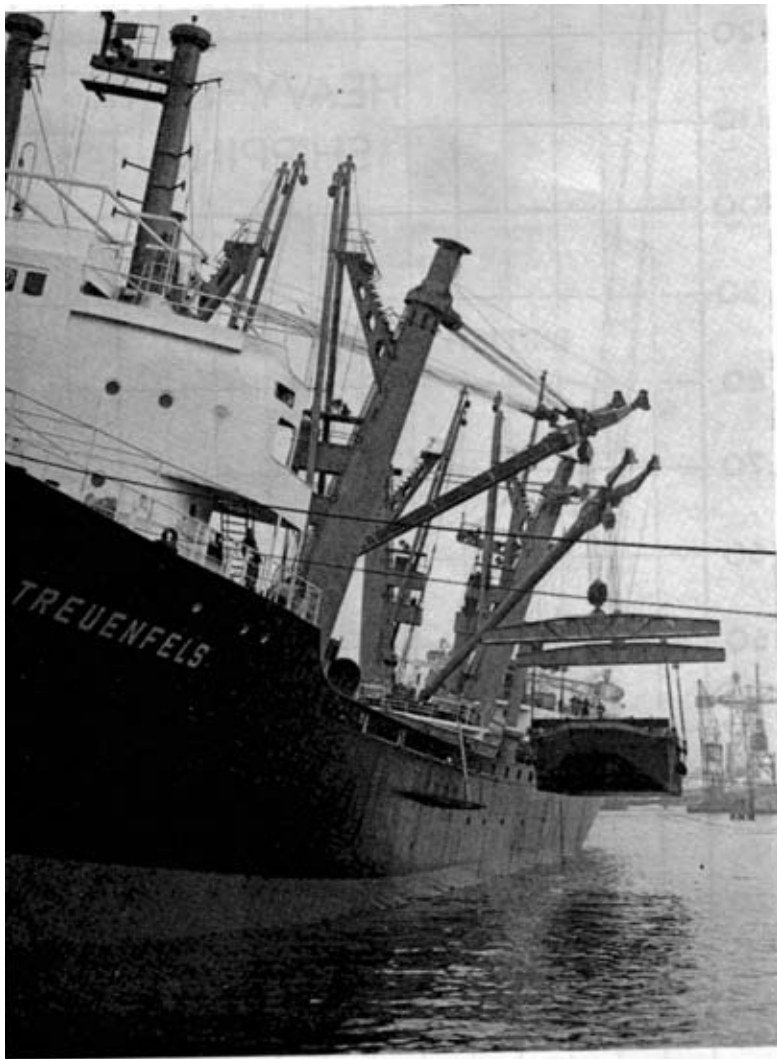
Photo 6. A 269-ton test load being lifted by the two Stülcken derricks (each 130-ton SWL) of the Hansa liner Treuenfels , working in tandem. When lifting a craft out of water, an initial loss in pull, due to suction, must be allowed for. (By kind permission of H. C. Stülcken of Hamburg.)
