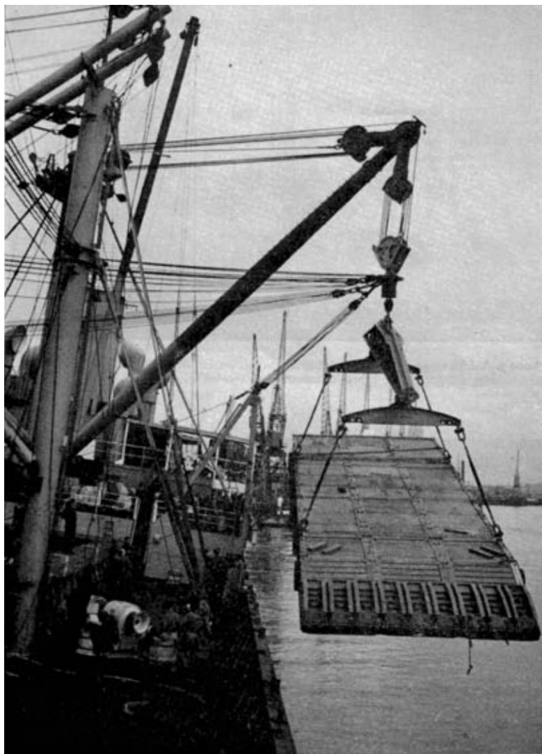
Photo 5. A 60-ton NL pontoon ferry for Christmas Island is lifted aboard the Benueyis using her 120-ton derrick. Note the use of the lifting beam and spreader arms, and also the power guys which enable the load to be pulled horizontally with the least strain on the derrick.
