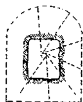
RING DRILLING TO ENLARGE HEADING TO FULL SIZE.
