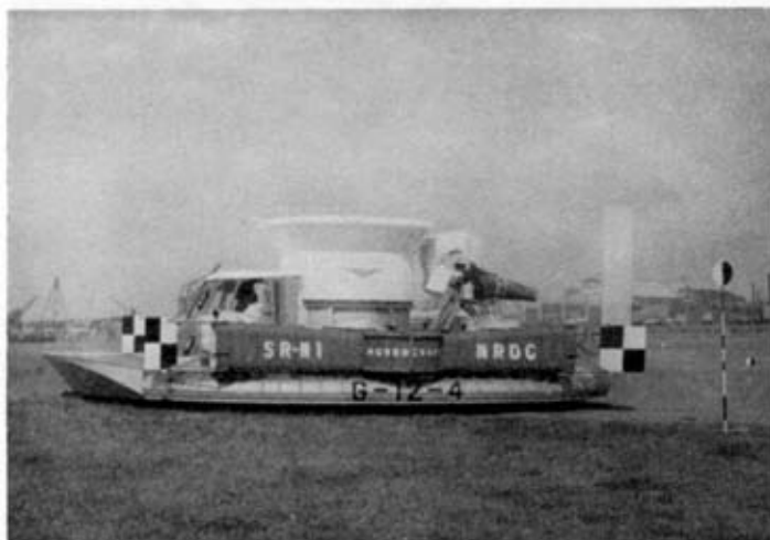
Photo 4. The SRN 1 Hovercraft coming ashore on Upnor Hard. Note the additional jet engine mounted at the stern for greater forward speed
